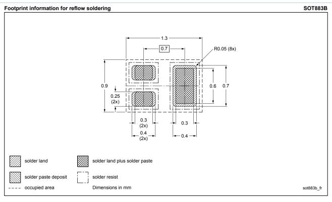
Fig. 20. Reflow soldering footprint for SOT883B (DFN1006B-3)
