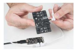
Grab another of the TRRS cables and plug it into the "Out" jack on the button board.
