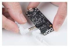
Take the other end of this cable and plug it into the audio jack of the phone, tablet, or computer that you'll be using to program the system.
