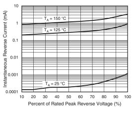
Fig. 4 - Typical Reverse Characteristics
