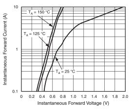
Fig. 3 - Typical Instantaneous Forward Characteristics
