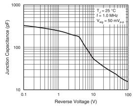
Fig. 5 - Typical Junction Capacitance
