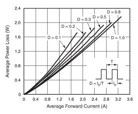
Fig. 2 - Forward Power Loss Characteristics
