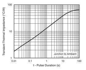
Fig. 6 - Typical Transient Thermal Impedance
