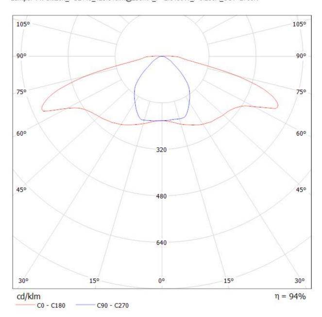
Luminaire: LEDiL Oy C14119\_STRADA-SQ-FS2\_(MK-R)+glass Eff.83.8% Lamps: 1 x Cree\_MK-R\_354.207lm@250mA\_CCT=3276K\_P=2.84547W\_l=249.8mA
