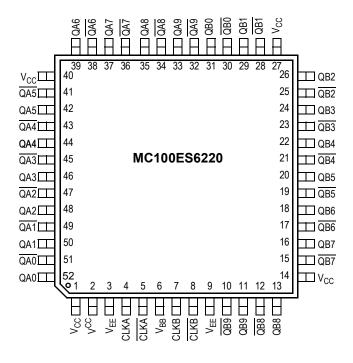
Figure 2. 52-Lead Package Pinout (Top View)
