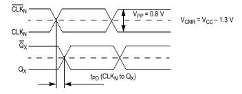
Figure 4. MC100ES6220 AC Reference Measurement Waveform
