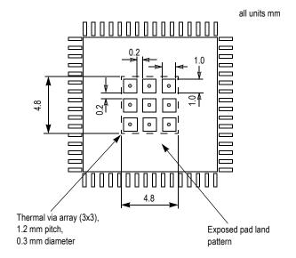
Figure 7. Recommended Solder Mask Openings
