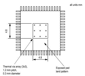
Figure 6. Recommended thermal land pattern
