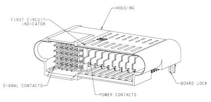
Front Connector View Looking at Blades and Pins (view looking in at rear of power supply)
