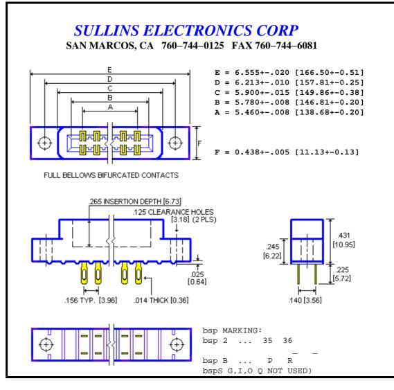
1.0 SPECIFICATIONS FOR A DUAL 36/72 POSITION EDGECARD CONNECTOR
