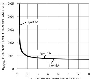
V<sub>GS</sub>, GATE-SOURCE VOLTAGE (V) Figure 4 Typical On-Resistance vs Drain Current and Gate Voltage
