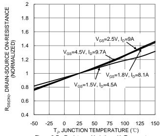
Figure 6 On-Resistance Variation with Temperature
