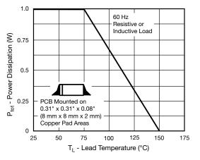
Fig. 1 - Maximum Continuous Power Dissipation
