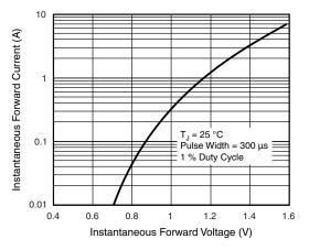
Fig. 3 - Typical Instantaneous Forward Characteristics
