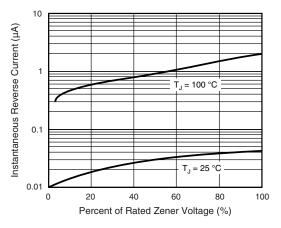
Fig. 4 - Typical Reverse Characteristics
