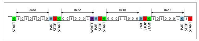
Figure 22: Example of Read (Reg[0x2B], Reg[0x2C])
