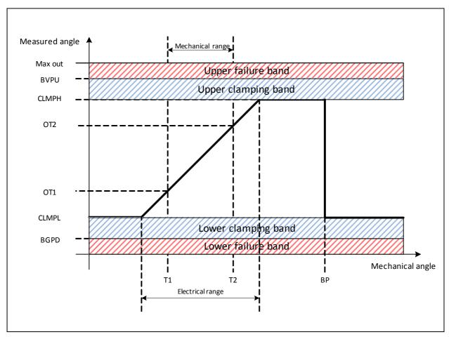
The breakpoint BP sets the discontinuity point where the output jumps from one clamping level to the other. It is strongly recommended to set the breakpoint at the maximum distance from the start and stop position (T1 and T2). To handle the case of a full turn, a hysteresis function across the breakpoint can be used to avoid sudden jumps between the lower and upper clamping level.
