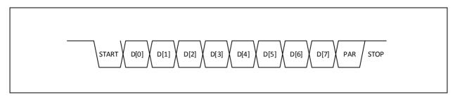
The PAR bit is even parity calculated over the data bits (D[0:7]). Each frame is transferred from LSB to MSB.
