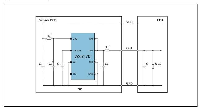
Figure 43 and Figure 44 show the recommended schematic in the application. All components marked with (\*) are optional and can be used to further increase the EMC.
