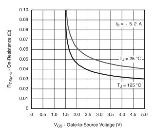
On-Resistance vs. Gate-to-Source Voltage
