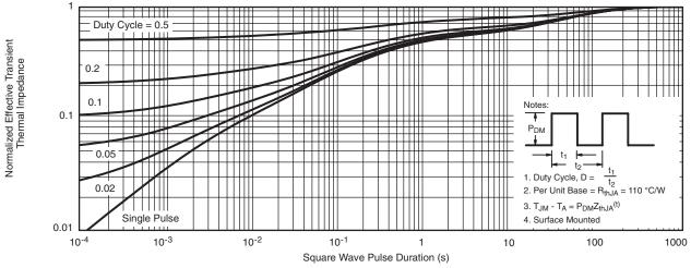
Normalized Thermal Transient Impedance, Junction-to-Ambient
