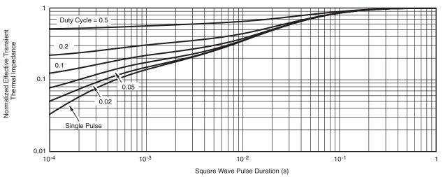
Normalized Thermal Transient Impedance, Junction-to-Foot
