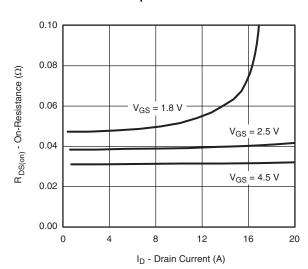
On-Resistance vs. Drain Current and Gate Voltage
