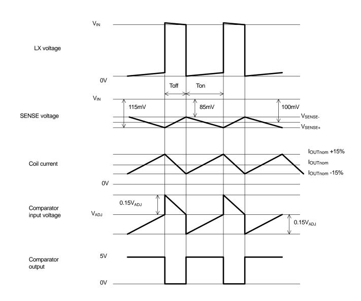
**Figure 2. Operating Waveforms**
