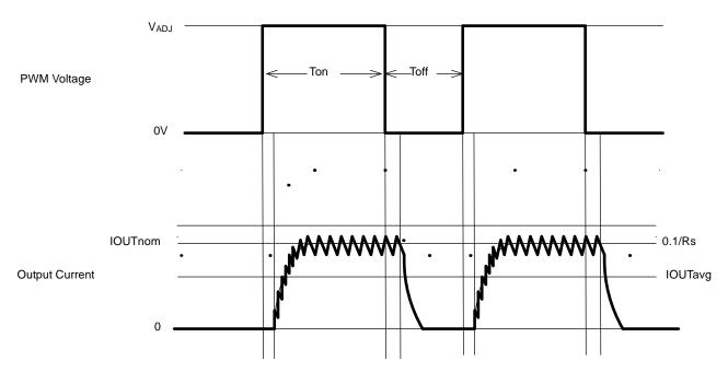
Figure 3. Low Frequency PWM Operating Waveforms
