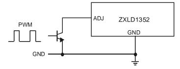
This scheme uses the 50k resistor between the ADJ pin and the internal voltage reference as a pull-up resistor for the external transistor eg MMBT3904.
