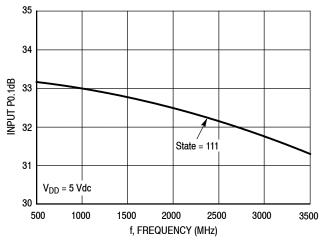
Figure 12. Input P0.1dB versus Frequency
