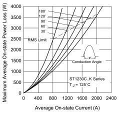
Fig. 5 - On-State Power Loss Characteristics
