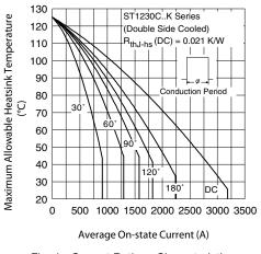
Fig. 4 - Current Ratings Characteristics
