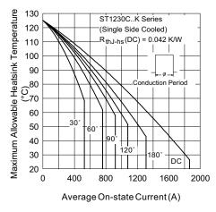
Fig. 2 - Current Ratings Characteristics
