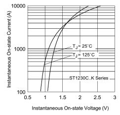
Fig. 9 - On-State Voltage Drop Characteristics
