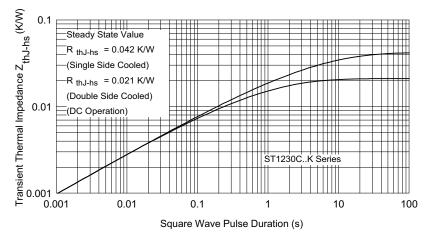
Fig. 10 - Thermal Impedance Z<sub>thJ-hs</sub> Characteristics
