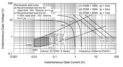
Fig. 11 - Gate Characteristics
