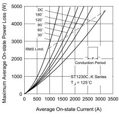
Fig. 6 - On-State Power Loss Characteristics
