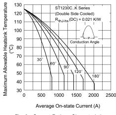
Fig. 3 - Current Ratings Characteristics
