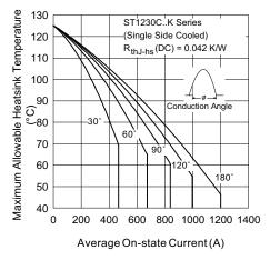
Fig. 1 - Current Ratings Characteristics
