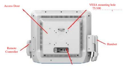
Rear I/O connectors (power jet LAN/USB port 2-pin phoenix)
