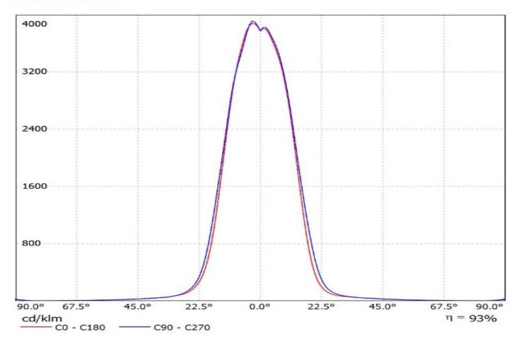
Luminaire: Ledil Oy CA11138\_LC2-M\_(XR-E)\_SIMULATED Lamps: 1 x Cree XR-E
