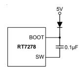
Figure 5. External Bootstrap Diode
