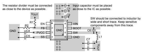
Figure 7. PCB Layout Guide
