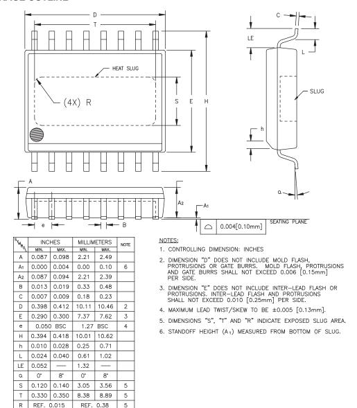
Figure 4: Package Outline - 16 Pin Wide Body SOIC with Heat Slug
