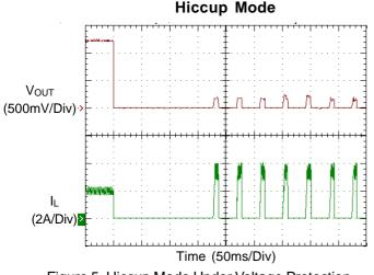
Figure 5. Hiccup Mode Under Voltage Protection
