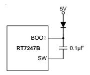
Figure 2. External Bootstrap Diode
