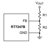
Figure 1. Output Voltage Setting
